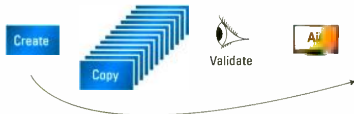
Figure 1. There are four basic steps common to contemporary graphics workflows: creation, versioning (copy), verification (validate) and playout (air).
